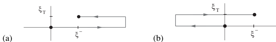
Figure 7.12. The gauge link structure in the quark-quark correlator \Phi in SIDIS (a) and Drell-Yan process (b) respectively.
